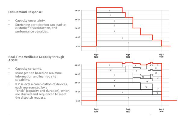
Unique capacity profiles are represented by dispatch "bricks," which are stacked and sequenced to meet the dispatch request. Each brick represents the unique capacity (height of brick associated with the Y axis) and duration of control capability (length of brick associated with the X axis).
