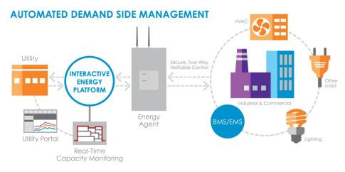
BMS: Building Management System EMS: Energy Management System HVAC: Heating, Ventilation, Air Conditioning
